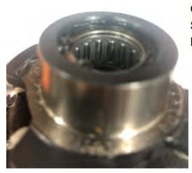
Caged Needle Roller Bearing fitted to the Load Sprocket brake assemble side which supports the Pinion Drive Shaft.
